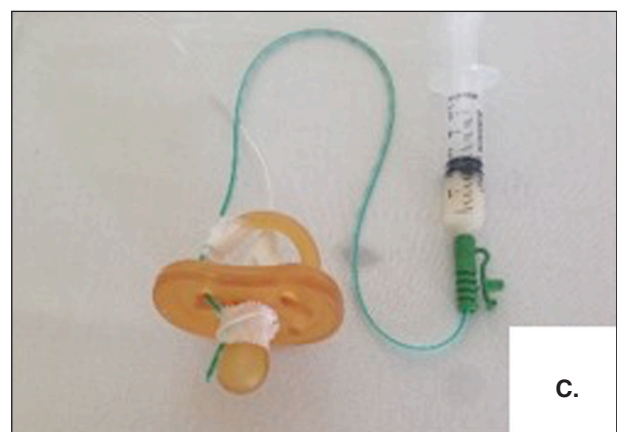
Figure 1. A. Prototype with the pacifier connected to the pressure sensor and BIOPAC A/D converter. B. Pacifier adaptation for non-nutritive sucking (NNS) measurement. C. Pacifier adaptation for nutritive sucking (NS) measurement.
