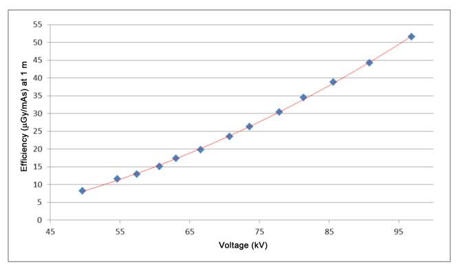
Figure 2. X-ray tube output curve.
