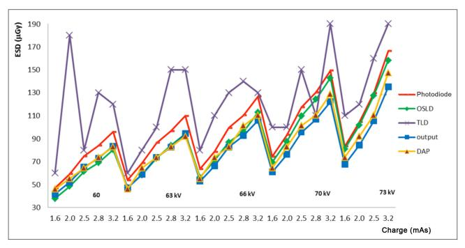
Figure 1. Comparison of Entrance Skin Dose (ESD) measurement with different methods.
