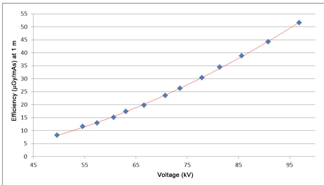
**Figure 2.** X-ray tube output curve.
